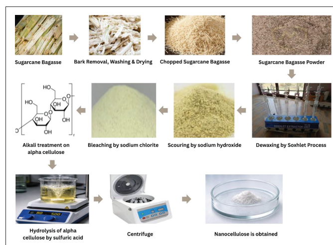
Figure 2 : Synthesis of nanocellulose powder.
