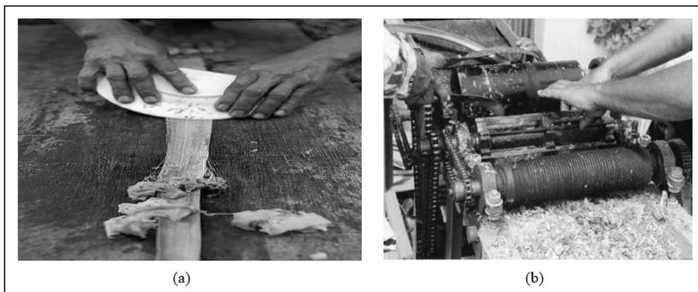
Figure 4: (a) Manual extraction and (b) Mechanical extraction of PALF [56].
