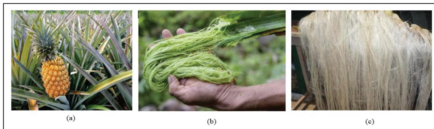
Figure 2: (a) Pineapple Plant with Fruit (b) Extracted PALF (c) Raw PALF
